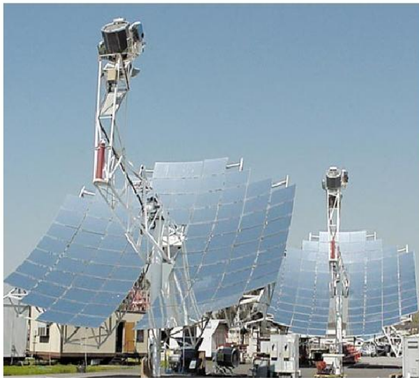
25-kWe Boeing/SES Dish-Stirling Systems on test in Huntington Beach, CA
